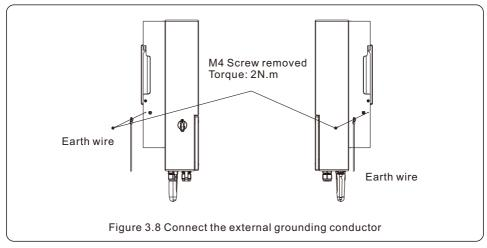
To connect the grounding terminal on the heat sink, please follow the steps below:
