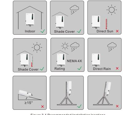
Figure 3.1 Recommended Installation locations
