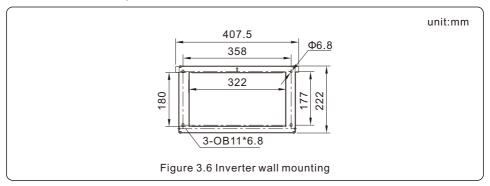
Once a suitable location has be found accordingly to 3.1 using figure 3.6 mount the wall bracket to the wall.
