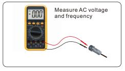
Step 2: Turn on the OCPD for the system and then measure the AC voltages line to line and line to neutral. The backup side of the system will be off until commissioning is complete. Turn the OCPD back off for now.
