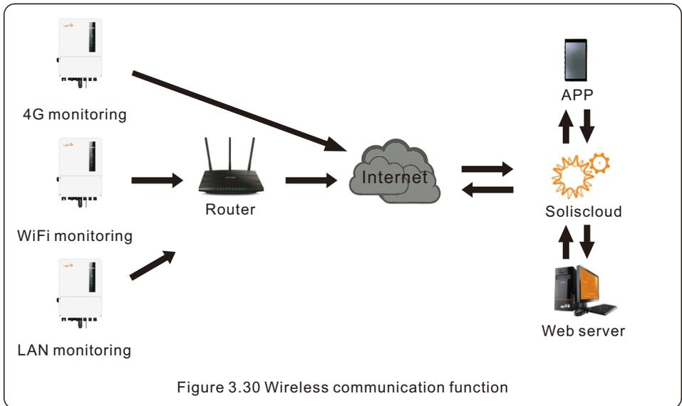
Figure 3.30 Wireless communication function
