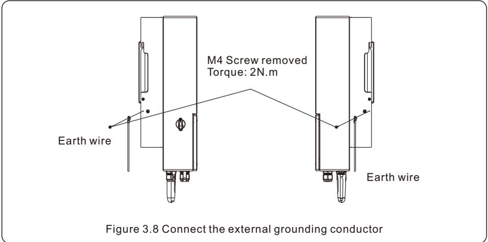
Figure 3.8 Connect the external grounding conductor
