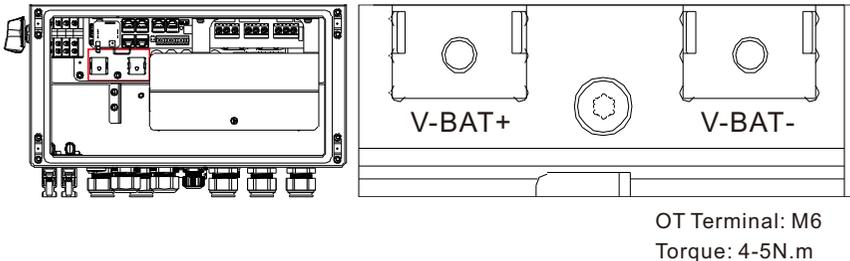
Figure 3.17 Battery cable connection
