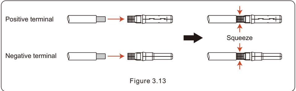
5. Insert the crimped DC cable into the DC terminal firmly, then insert the waterproof rubber ring into the DC terminal and tighten the nut.
