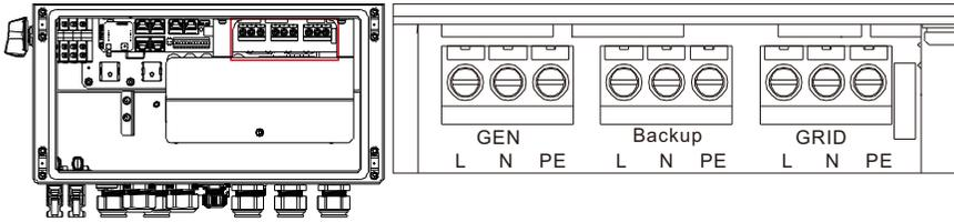
Figure 3.18 AC output terminals
