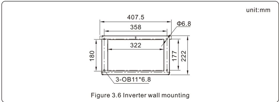
Figure 3.6 Inverter wall mounting
