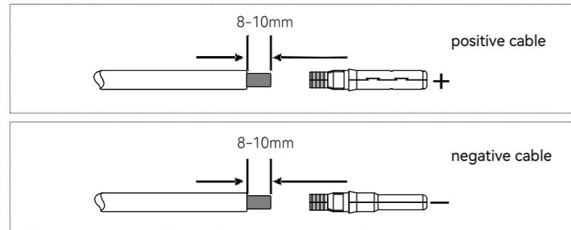
3. Assembly the positive and negative cables with corresponding crimping pliers.
