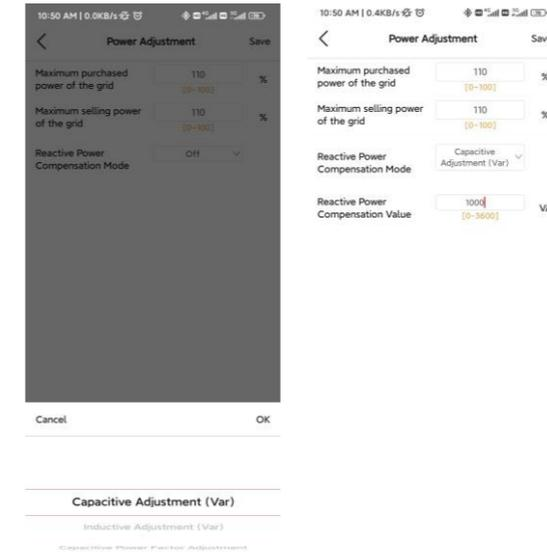
Step 1: Select Inductive Adjustment Var or Capacitive Var according to your local grid regulation. The power range is from -60%Pn ~ 60%Pn.
