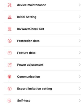
Step 3: You can choose self-test item required. Individual self-test time is approx. 5 minutes. All self-test time is approx. 40 minutes. After the self-test is completed, you can save the test report. If self-test is failed, please contact with SAJ or your inverter supplier.
