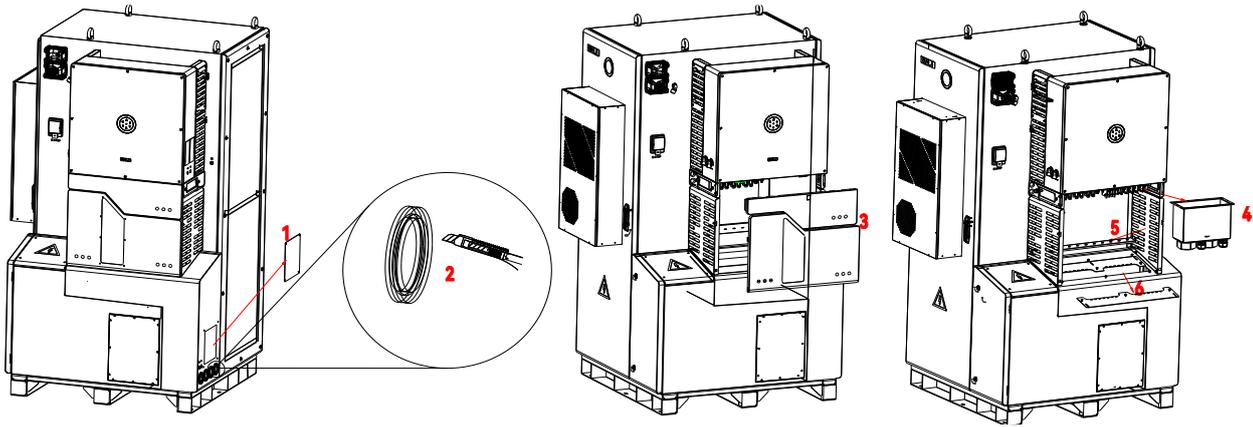
Note: The machine and external wiring need to pass through the machine through the hole in the lower right corner of the machine.
