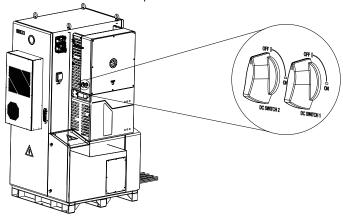
7. Connect the positive and negative connectors into positive and negative DC input terminals of the inverter, a "click" should be heard or felt when the contact cable assembly is seated correctly.
