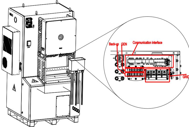
3. Secure all parts of the grid and backup connector tightly.
