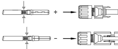
5. Fasten the lock screws on positive and negative connectors.
