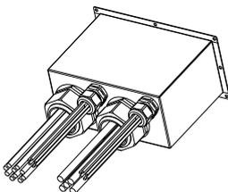
2. Connect the communication cable to the corresponding port. GRID, GEN and Back-up Fix the cables according to conductor marks of L1,L2,L3,N and PE.
