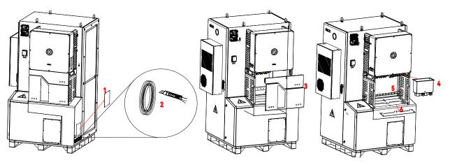
Note: The machine and external wiring need to pass through the machine through the hole in the lower right corner of the machine.
