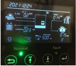
If with a neutral face icon, the inverter is in warning status. The code after the neutral face is a warning code. If a sad face icon is showing, the inverter is in fault status. The code represents the error code. Please refer to the troubleshooting chapter of the user manual for the meaning and countermeasures of the warning code and error code.
