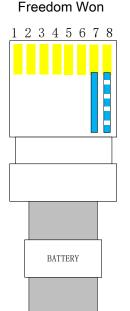
Battery Pin out: PIN1: NC PIN2: NC PIN3: NC PIN4: NC PIN5: NC PIN6: NC PIN7: CAN H PIN8: CAN L
