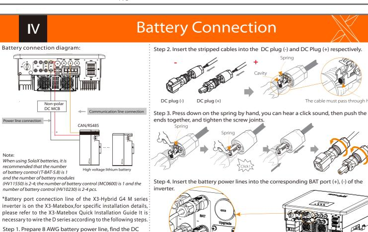
Note: The positive and negative wires of the battery are not allowed to be reversed! Note!
