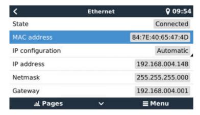
When using Ethernet and State shows 'Unplugged', verify that the Ethernet network cable is not faulty: try another one. The two lights at the back of the Cerbo GX, where the Ethernet RJ45 cable plugs in, should be lit or blinking. Two dead lights indicate a connection problem.
