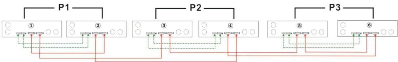
Three inverters in one phase, two inverters in second phase and one inverter for the third phase:
