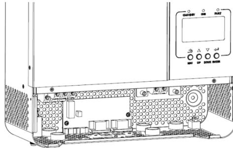
**Step 6:** Re-connect 2-pin and 14-pin to original position.
