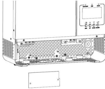
**Step 4:** Remove two screws as below chart to take out cover of parallel communication.
