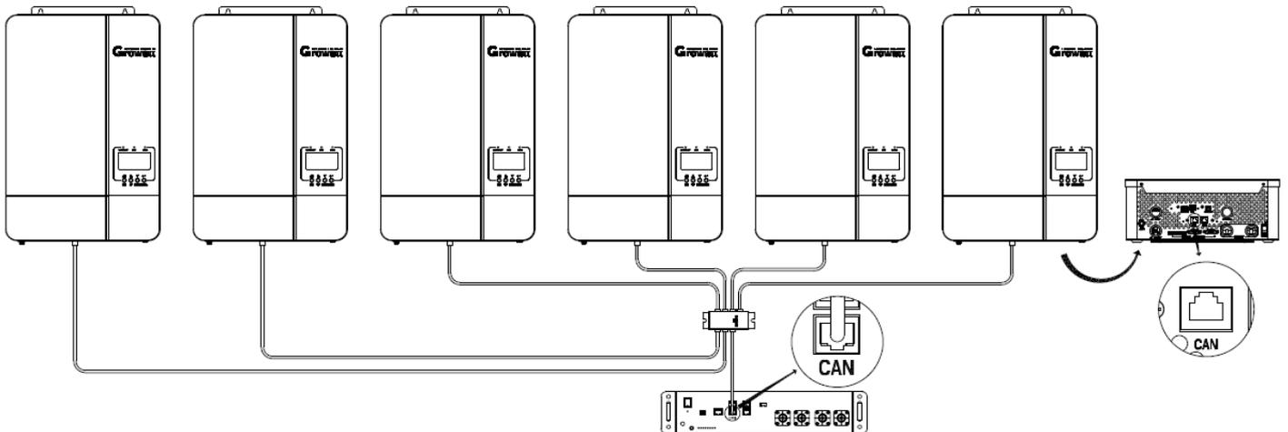
**Note:** if inverters parallel as 3 phase system, only need to connect L1-Phase inverters with lithium battery RJ45 port to communicate with BMS. When inverters on L1-Phase are more than 2 units, it would need an extra RS485/CAN HUB to converge inverters on L1-Phase to connect with battery RJ45 port to communicate with BMS.
