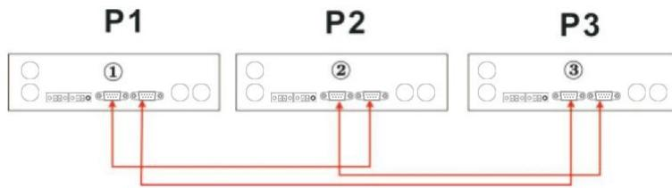
Two inverters in one phase and only one inverter for the remaining phases:
