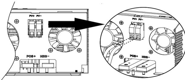
connectors. Then, connect positive pole (+) of connection cable to positive pole (+) of PV input connector. Connect negative pole (-) of connection cable to negative pole (-) of PV input connector.
